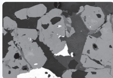
Backscattered SEM image of polished Granite
